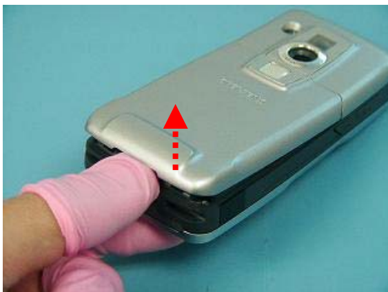
Remove Battery cover.
