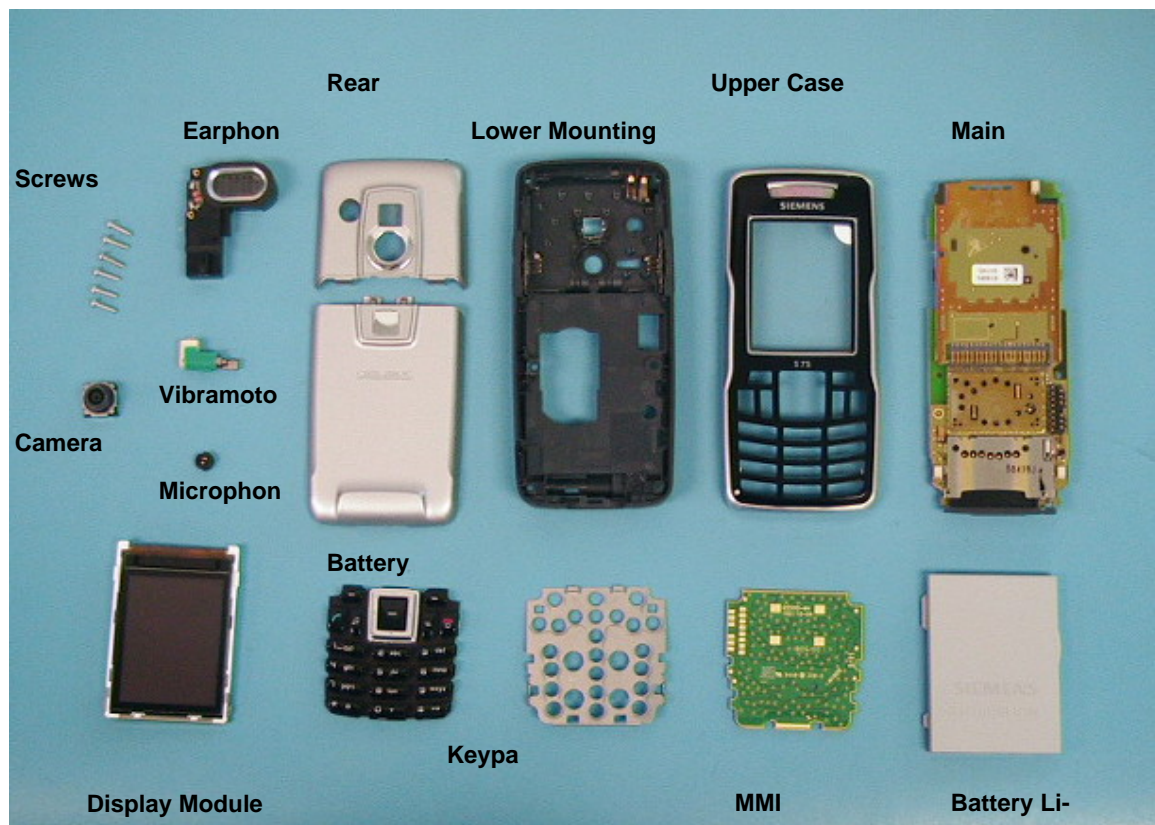
Fully disassembled S75
